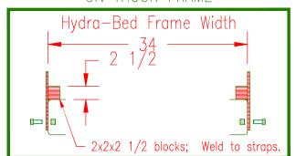
Bolt 2 1/2x2 1/2x38 3/4" tube to factory frame riser using 1/4X2X3 reinforcing plates. Center Hydra—Bed between the tube risers. Weld Hydra—Bed to tube risers. Hydra—Bed frame will be resting on the tube and between risers.
